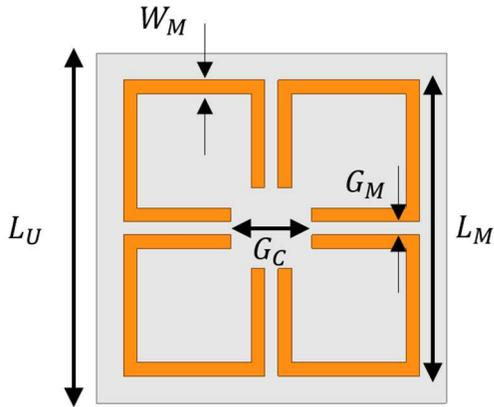
Fig. 3. Top view of the MTM unit cell, where  $L_U = 27.5 \text{ mm}$ ,  $L_M = 23.5 \text{ mm}$ ,  $W_M = 1 \text{ mm}$ ,  $G_M = 1 \text{ mm}$ ,  $G_C = 6 \text{ mm}$ .
