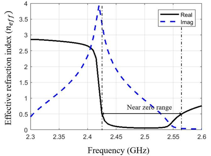
Fig. 4. Simulated effective refractive index of the MTM unit cell.
