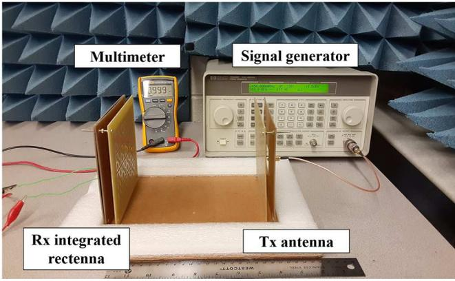
Fig. 12. Measurement setup for the proposed 3D integrated rectenna.
