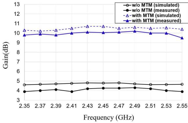
Fig. 9. Simulated and measured peak gain of the patch antenna without and with MTM.
