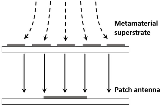
Fig. 2. Conceptual principle of gain improvement in a patch antenna using an MTM superstrate.
