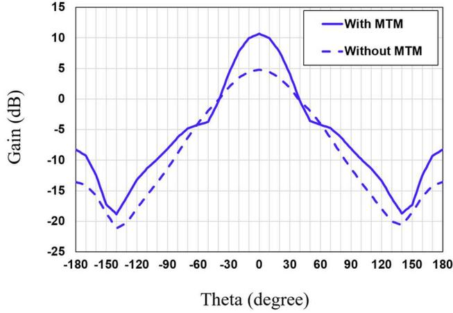
Fig. 8. Simulated radiation patterns of the patch antenna with and without MTM superstrate at 2.45 GHz.
