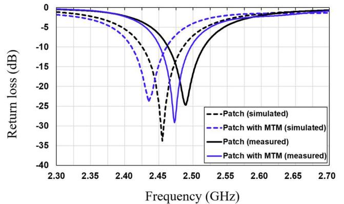
Fig. 7. Simulated and measured return loss results of the patch antenna without and with MTM superstrate.
