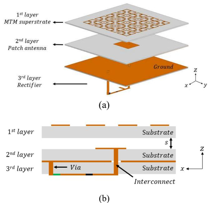
Fig. 1. Schematic of a 3D integrated rectenna: (a) perspective view, (b) side view, where  $s = 10 \text{ mm}$ .
