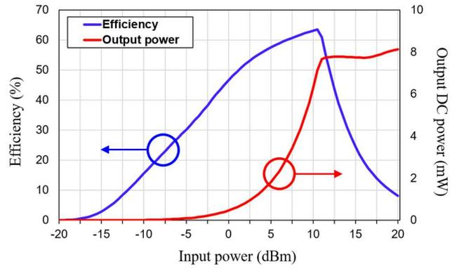
Fig. 13. Measured RF-DC conversion efficiency of the 3D integrated rectenna.
