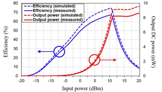
Fig. 11. Simulated and measured RF-DC conversion efficiency of the rectifier circuit.
